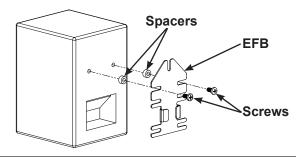
Slide the Speaker and EFB onto the L-Bracket on the stand.
